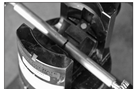
FIGURE 7a: Slide sleeve over one conductor so it protrudes out the end.
