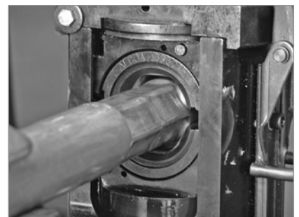
FIGURE 11b: Overlap each compression by 1/4 inch (6.4 mm).
