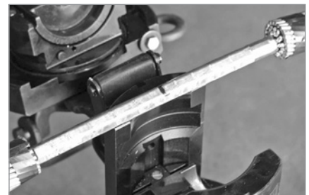
FIGURE 7b: Overlap each compression on Steel sleeve 1/4 inch (6.4 mm).
