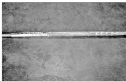
FIGURE 11c: Completed compression splice.
