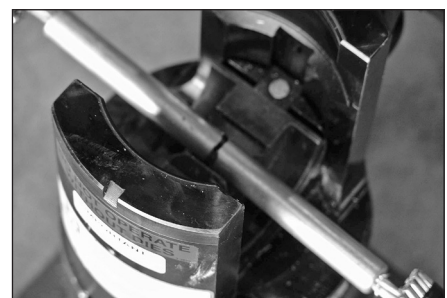
FIGURE 6: Slide sleeve over one conductor so it protrudes out the end.
