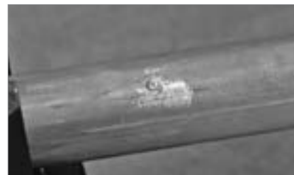
FIGURE 10c: Peen edge of filler hole over top surface of plug.
