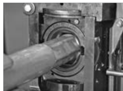
FIGURE 11b: Overlap each compression by 1/4 inch (6.4 mm).
