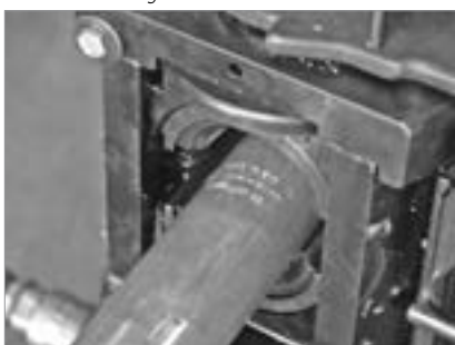
FIGURE 11a: Make the initial compression at the "start" mark.
