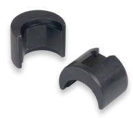
The 30 Ton AH and SH Dies are designed to compress Standard Compression Accessories and HiTemp™ Compression Accessories. The 30 Ton CD Dies are designed to compress Quick Compress<sup>®</sup> Accessories. These dies are to be used with the Model 30 A press.
