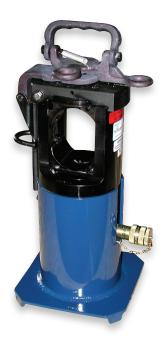
The 60AGSC and 60AFTGSC presses are portable 60-ton construction and maintenance tools designed to cover a full range of compression accessories requiring die sizes up to and including 40AH. The 60AFTGSC features an integral hinged head with eyes suitable for hot line work.
