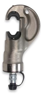
AFL's Model 30A Hydraulic Press is a proven, single-acting hydraulic tool designed for installing connectors with 30 tons of force at 10,000 psi (68.9 MPa).
