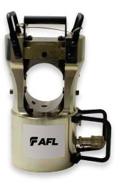
The 100A Single or Double Acting Press is designed for the installation of compression fittings. The 100A develops 100 tons of force at 10,000 PSI. A special piston facilitates operation in single or double acting mode. Redesigned for portability, the press now weighs 95 pounds.
