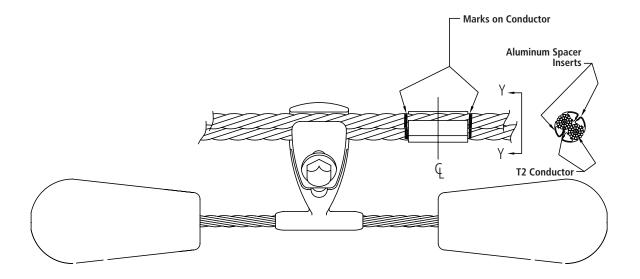
NOTE: 1700-T2 Dampers are only for use on overhead transmission line twisted pair cables.
