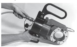
**5.** Slide the head assembly on to the power unit and ensure the rollers on the die block roll into place. (**Note:** Incorrect assembly could damage the tool and dies when compressed. Ensure your press head is aligned with the power unit.)
