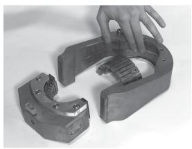
**2.** With the die faceplate off, slide die into grooved area of the head ensuring it sits correctly in the bottom faceplate.
