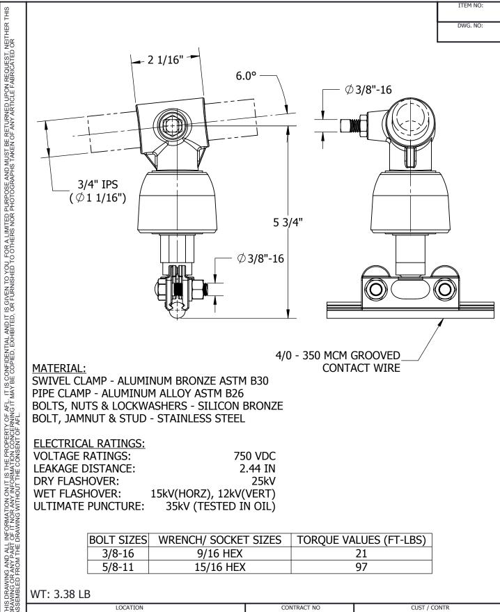
**BOLTS, NUTS & LOCKWASHERS - SILICON BRONZE BOLT, JAMNUT & STUD - STAINLESS STEEL**
