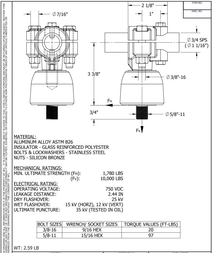
**ALUMINUM ALLOY ASTM B26 INSULATOR - GLASS REINFORCED POLYESTER BOLTS & LOCKWASHERS - STAINLESS STEEL NUTS - SILICON BRONZE**
