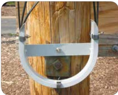
The AFL DCSU Fiber Storage Unit is designed to store and organize the slack from a fiber drop that is left at a fiber distribution terminal. The DCSU can also be used for the organization or storage of any unused multi-fiber drop in the placing of a multi-port terminal from VATS splices. In this way, cable left for future use is safely stored. The DCSU can manage up to 12 fiber drops when laid flat into the raceway, with minimal slack required at the terminal.
