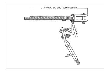
The 33200 Series Dead End Assembly is specifically designed for AWAC conductors. The aluminum body of the dead end is fabricated from AFL seamless drawn aluminum. The tongue and terminal pad are constructed with a 15° angle, which permits the terminal connector to be bolted in the straight or 30° position.
