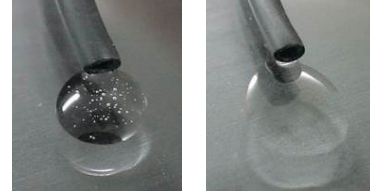
Bubble Separator Performance
