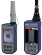
**FOCIS Flex and FOCIS Lightning (Multi-Fibre) Connector Inspection**
