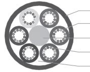
Insect Resistant Nylon Moisture Resistant Jelly Filled Loose Tube Central Strength Member Optical Fibre
