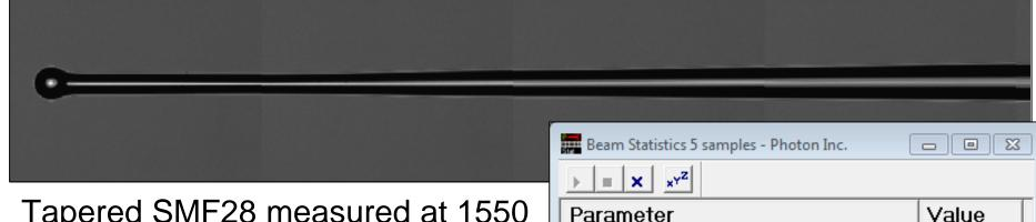
Tapered SMF28 measured at 1550 nm. Fiber end curvature radius = 50 um. Incident angle ≈ 16°
