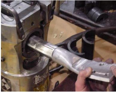
Press the Terminal Connector over the conductor. Make the initial compression at the start knurl. Continue making compressions to the end of the Terminal Connector barrel, **overlapping the previous compression by approximately 0.50 inches (1.27 cm). Complete die closure is required for each compression.**
