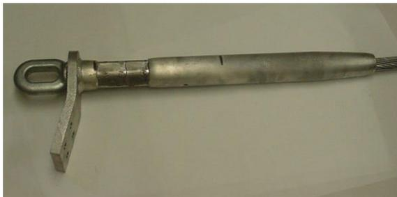
Make initial compression on the dead end body over the steel shank beginning at the start knurl nearest the dead end tongue. Continue making compressions to the stop knurl, **overlapping the previous compression by approximately .50 inch (1.27 cm). Complete die closure is required for each compression.**
