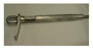
Make initial compression on the dead end body over the steel shank beginning at the start knurl nearest the dead end tongue. Continue making compressions to the stop knurl, **overlapping the previous compression by approximately .50 inch (1.27 cm). Complete die closure is required for each compression.**
