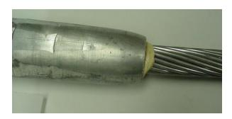
Filler Compound should be visible at end of the barrel during the final compressions (if adequate amount has been pumped in).
