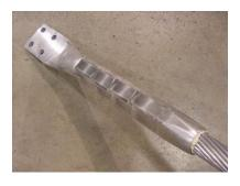
Filler Compound should be visible at end of the barrel during the final compressions (if adequate amount has been pumped in). Compressed portion of the Terminal Connector should have a smooth uniform appearance. Remove flash, if present, with file or emery cloth. Clean contact surface of Terminal Connector and Dead End pad.
