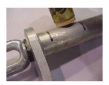
Lubricate area to be compressed from "Start" knurl to "Stop" knurl as illustrated.
