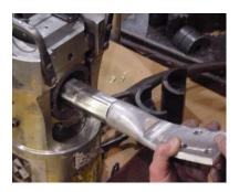
Press the Terminal Connector over the conductor. Make the initial compression at the start knurl. Continue making compressions to the end of the Terminal Connector barrel, **overlapping the previous compression by approximately 0.50 inches (1.27 cm). Complete die closure is required for each compression.**
