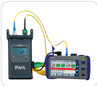
Multi-fibre Switch paired with FlexScan® OTDR
