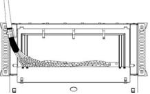
2: Route the prepared cable through the back of the patch panel. Secure the incoming cable with the cable clamp.
