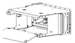
1: From the rear of the XFM panel, remove the tray cable guide from the base plate and reattatch it to the top of the panel. The tray's two plungers may be used to remove and secure the tray.
