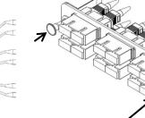
5: Attach the adapter plate to the module base by pressing in the nylatch plungers.
