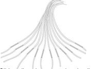
2: Slide splice sleeves on the pigtails.
