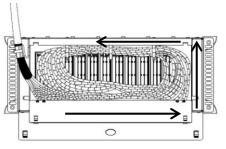
4: Route the cable slack through the cable routing guides in the back of the panel.
