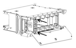
3: Install all modules from the front of the panel by pressing in the nylatch plungers.
