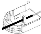
2: Mount the incoming fiber into the module using the mounting clip. The fiber may enter from either side of the module, so the most convenient mounting position may be selected.
