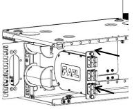
2: Install the first module into the panel by pressing in the nylatch plungers.
