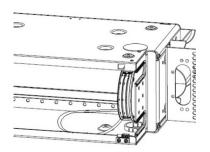
3: Route the cable slack in a 6 <sup>3</sup>/<sub>4</sub>" diameter circle beneath the module.
