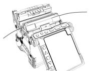
4: Splice Fibers. Position splice sleeve over exposed fiber and use heater to shrink the sleeve. Repeat for all matched incoming and pigtail fibers.
