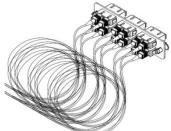
1: Organize the prepared incoming fiber and pigtails on a suitable work surface.
