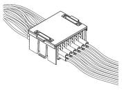
6: Attach the splice holder assembly cover once all the splice sleeves have been inserted.
