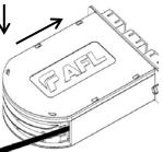
6: Place the plastic cover onto the module and slide it forward to lock it into place.
