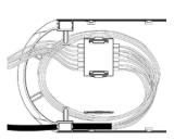
3: Starting at the mounting clip, route the incoming fiber into the module. Create 1.5 loops around the bottom of the housing. Mount the splice sleeve holder on the module base.
