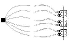
3: Prepare matched incoming and pigtail fibers for splicing: Strip, Clean, and Cleave. Then secure the prepared fibers in the splicer.
