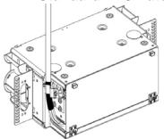
1: Route the prepared cable through the back of the patch panel. Secure the incoming cable with the cable clamp.
