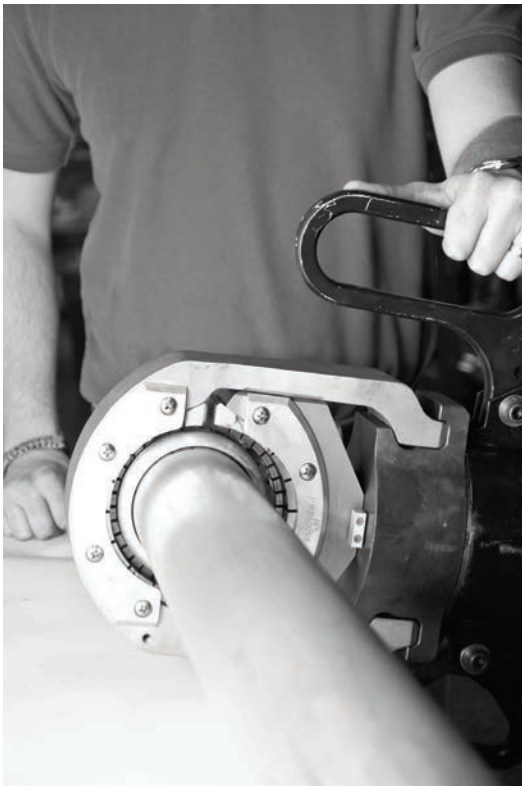
Fig. 7—NOTE: ALWAYS PROPERLY POSITION YOURSELF TO THE SWAGE PRESS WHEN COMPRESSION IS IN PROGRESS. KEEP CLEAR OF THE PRESS HOSE. SEE FIG. 7.
