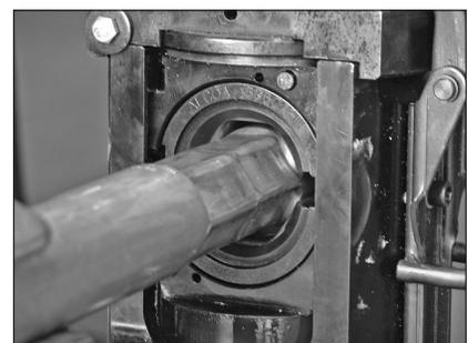
FIGURE 11b: Overlap each compression by 1/4 inch (6.4 mm).
