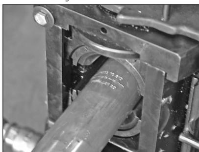
FIGURE 11a: Make the initial compression at the "start" mark.
