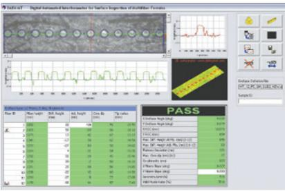
Interferometer view of MTP connector end face geometry
