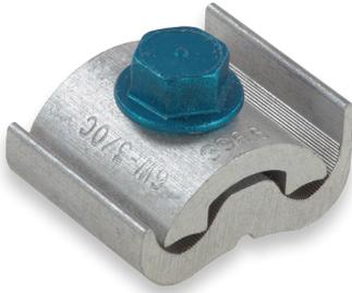
Catalog 390 and Catalog 490 Series Distribution Parallel Groove Clamps with a single bolt accommodate a range of conductors in each groove. This type of clamp is commonly used for service drop connections and as a tap from large to relatively small conductors.
