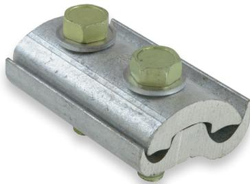
Catalog 480 Series Center Bolt Clamps are a multiple bolt heavy duty universal groove design which can handle the full electrical load of the conductor. They offer the convenience of installation without any loose parts. Catalog 480 Clamps are made from extruded high strength aluminum alloy and can be taped easily. Additionally, they have a minimum bulk, which results in a neat appearance.
