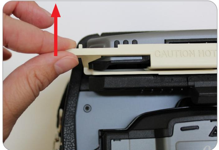
Figure 10. Lift heater out by handles
