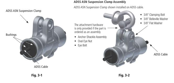
7. Install ADSS ASN Suspension Clamp Assembly to Oval Clevis Eye or other attachment hardware. Make final visual inspection on ADSS ASN Suspension Clamp to ensure that the assembly (groove-bushings) are not cocked or misaligned, but properly seated.
