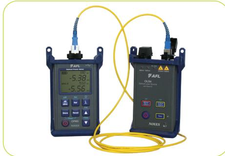
SMLP5-5 Optical Loss Test Kit
