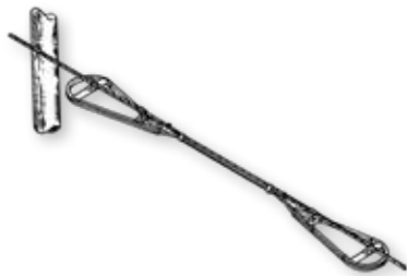
Reserve Cable Storage
