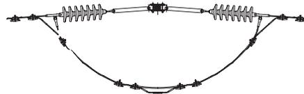
FIG. 2 – Tension Bypass
