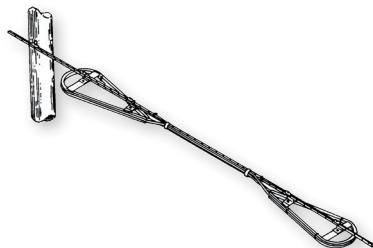
Reserve Cable Storage
