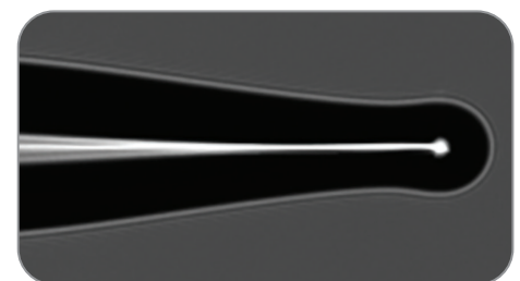
Tapered Probe with Small Ball End
