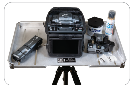
Worktray conveniently holds all necessary splice equipment
