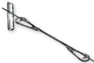
Reserve Cable Storage
