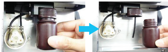
Resin and pump exchange
