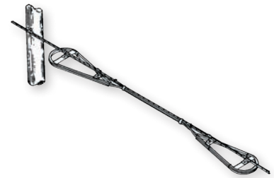
Reserve Cable Storage
