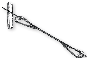
Reserve Cable Storage
