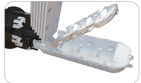
Open to access Apex X-3 splice trays and lock at 72 degrees
