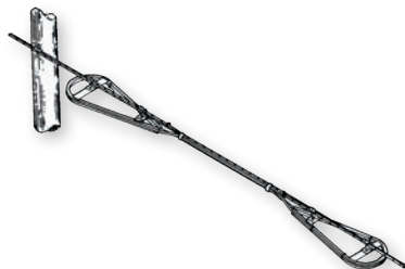
Reserve Cable Storage
