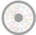
Typical 432 Fiber OSP Cable Construction
