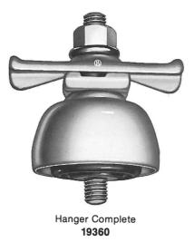
Type AGC tangent hangers consist of a replaceable Dirigo insulator housed in a metal shell, forming an air gap so spaced that flashover will take place at a voltage considerably below the dielectric strength of the insulator and yet high enough to prevent flashover from surge voltages of a magnitude generally encountered in street railway service. This hanger has excellent leakage characteristics because of the dry spot secured by the long overlap of the hanger shell.
