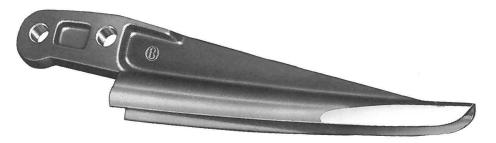
Lips have a 3½-inch taper at side and bottom to provide an easy transition of the carbon shoe from wire to runner. Narrow cross section affords ample side clearance. Construction of lips makes smooth peening possible and easy.
