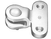
This yoke can be applied to advantage in installing all types of segments in span construction, attaching to the two outside pulloff Hi\*Lite strains as shown in accompanying drawing. It serves to space these insulators apart, equalizing strain on each. Time required to install is reduced and appearance improved.
