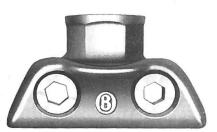
Two hollow screws tighten jaws which grip wire tightly. Jaws are 3-inches long, 1%-inches high, boss %-inch. Jaws and boss are cast of malleable iron, hot-dip gal-vanized. Hollow screws are made of bronze.
