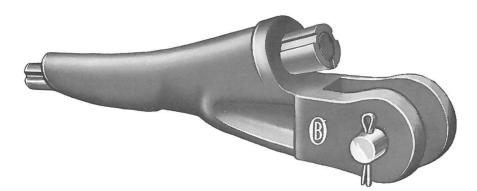
For deadending round or grooved contact wire. Made of bronze with stainless steel chuck for holding wire in place. Chuck is serrated on inside to give grip on wire and tapered on outside to fit into a tapered hole in body. Clevis fitted with  $\frac{1}{2}$ -inch rivet, hot-dip galvanized, and cotter. Clevis opening,  $\frac{13}{16}$  inch.
