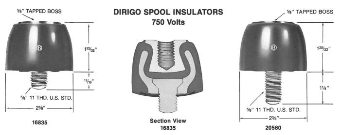
**Use** – Well established as a basic insulating unit in many exacting industrial, mining and transit applications. Particularly suitable for crane work as it is available with two different lower stud lengths. Used as secondary insulation with insulated hangers on grounded structures. Spool 16835 serves as the insulating unit in a number of O-B hangers.
