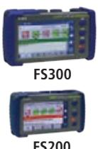
**FlexScan® FS300 (quad) and FS200 (single-mode) OTDRs**
