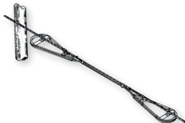
Reserve Cable Storage
