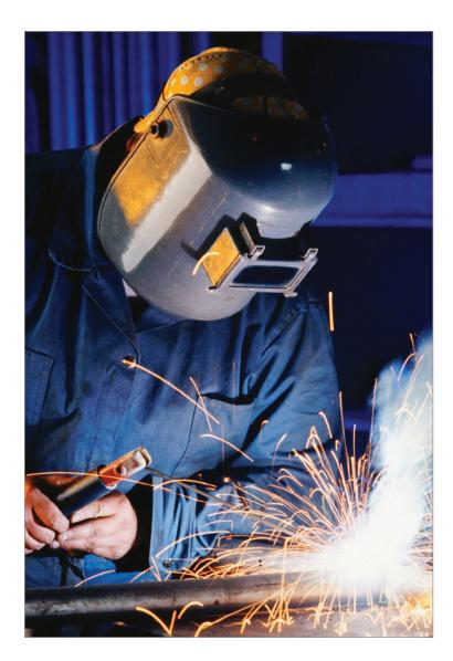
Welding of aluminum in electrical construction offers a superior and economical means of joining conductors. Electric arc welding using an inert gas shield produces mechanically and electrically sound joints requiring no flux or special surface preparation other than the cleaning of the surface to be welded.
