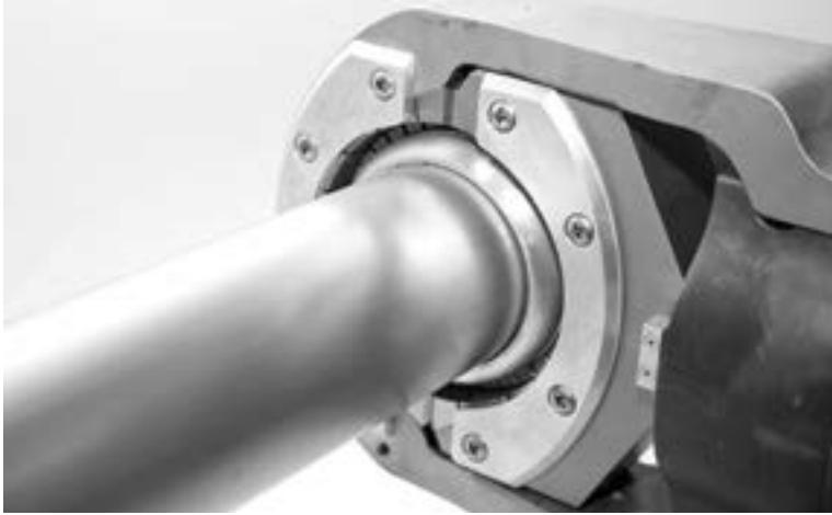
Fig. 6—NOTE: COMPLETE DIE CLOSURE IS REQUIRED ON ALL COMPRESSIONS.
