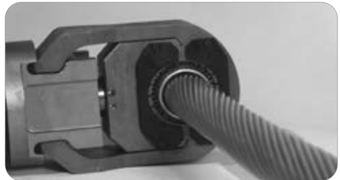
Fig. 4b—NOTE: Always properly position yourself to the Swage Press when compression is in progress. Keep clear of the press hose. See Fig. 6.
