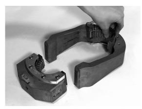
**3.** Install the top faceplate to lock the die into the head assembly using a Phillips head screw driver. Repeat steps for the die block assembly.
