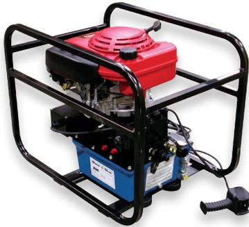
The 30GHR is a gas powered pump that produces 10,000 PSI of hydraulic pressure. The two-stage pumping system allows for rapid ram advance. The unloading pressure of the pump is 1,000 PSI. The 30GHR comes with a remote control with a 10 foot cord and is designed for continuous duty.
