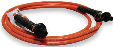
The 1/4" (0.635 cm) non-conductive, orange hose is made of an insulated, synthetic material. It allows a high flow rate for faster ram movement. Hoses are available with or without couplers for operating pressures of 10,000 PSI with a 4 to 1 burst ratio. Hoses are pre-filled with oil and pressure tested. The hoses are 3/8" NPT male thread on both ends and quick disconnects are 3/8" NPT female.
