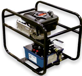
The 30GBM is a gas powered pump that produces 10,000 PSI of hydraulic pressure. It is designed to operate any 10,000 PSI compression tool. The two-stage pumping system allows for rapid ram advance. The “suc-o-matic” valve helps tools retract faster. The manual control has three settings: advance, hold and retract. The 30GBM is designed for continuous duty.
