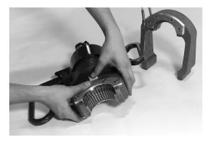
**6.** Remove safety caps from the bottom of power unit and the hose fitting. Insert hose fitting into power unit and tighten to ensure a tight seal.
