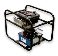
The 30GBM is a gas powered pump that produces 10,000 PSI of hydraulic pressure. It is designed to operate any 10,000 PSI compression tool. The two-stage pumping system allows for rapid ram advance. The "suc-o-matic" valve helps tools retract faster. The manual control has three settings: advance, hold and retract. The 30GBM is designed for continuous duty.
