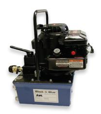
The 15GBM is a gas powered pump that produces 10,000 PSI of hydraulic pressure. It is designed to handle any high pressure tool up to and including the 60 ton press. The two-stage pumping system allows for rapid ram advance. The "suc-o-matic" valve helps tools retract faster. The manual control has three settings: advance, hold and retract. Whether making one crimp or 1,000 crimps, the 15GBM is the lightweight, portable answer.
