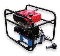
The 30GHR is a gas powered pump that produces 10,000 PSI of hydraulic pressure. The two-stage pumping system allows for rapid ram advance. The unloading pressure of the pump is 1,000 PSI. The 30GHR comes with a remote control with a 10 foot cord and is designed for continuous duty.
