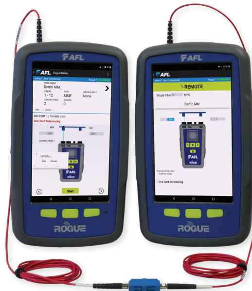
ROGUE OLTS Certifier kit with iB1 Bases
