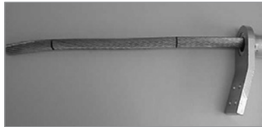
FIGURE 3: Slide aluminum dead end body over conductor.
