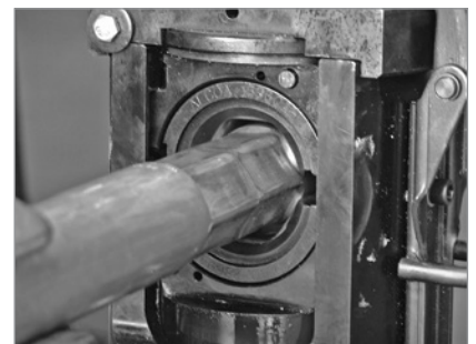
FIGURE 11b: Overlap each compression by 1/4 inch (6.4 mm).
