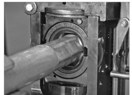
FIGURE 11b: Overlap each compression by 1/4 inch (6.4 mm).
