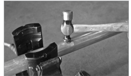
FIGURE 10a: Peen edge of filler hole over top surface of plug.
