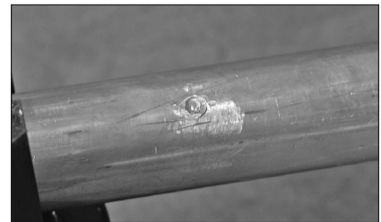
FIGURE 10c: Peen edge of filler hole over top surface of plug.
