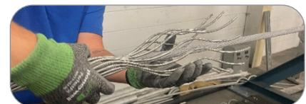
Figure 4 — Wrapping ends of inner rods
