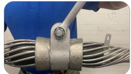
Figure 11 — Tightening bolt with wrench
