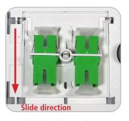
**6:** Then slide module out of retention slots.
