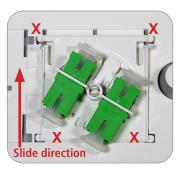
3: Align the four (4) tabs of module as shown to be locked into splice tray. Ensure all four (4) tabs are in place. Press down at the four **X** marks and slide forward to engage in the tray.
