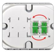
10: Rotate adapter frame 180 degrees (see Step 8) and the ferrules will meet off center and allow a larger boot on one side of the adapter frame.
