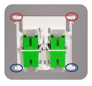
2: The reference tabs of the adapter module will be set in place where the blue circles are.
