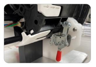
Figure 7 – Locking Clamp Engaged on Apex Base
