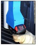
To remove battery, depress red tabs on side of battery and pull battery away from tool.
